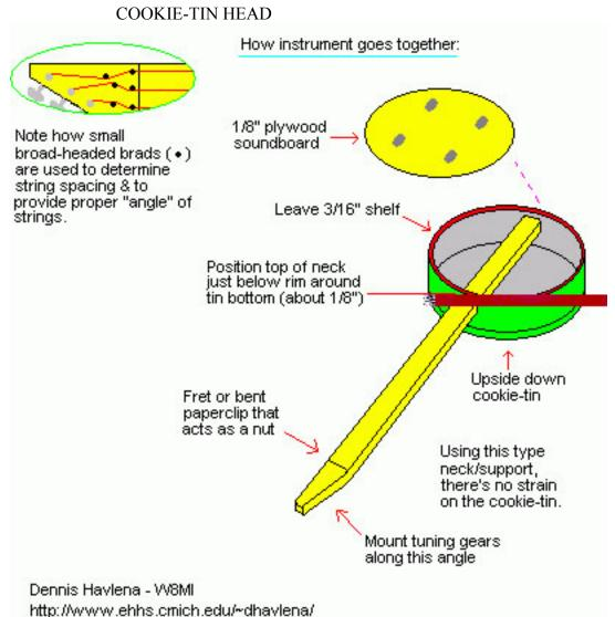
Although the tin-bottom will itself act as a fair resonator, a thin plywood sound-board greatly improves the tone and volume. Using a utility knife, cut a disk out of the bottom of the Cookie tin. Leave only about a 3/16" "shelf" remaining around the entire perimeter of the bottom. This is the ledge upon which the plywood sound-board rests.
