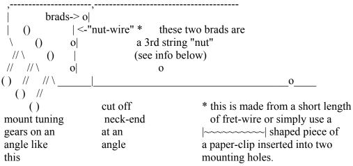
The three flat-headed brads nearest the tuning gears serve to determine the string spacing (there are no grooves in the "nut-wire") and to keep the strings pushed-down so that they pass solidly over the "nut-wire" without buzzing.
